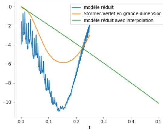
Figure 2.12: Variations of energy during time for solutions computed as in Figure 2.10. Solution of reduce model with hyper-reduction was computed for a longer time.
