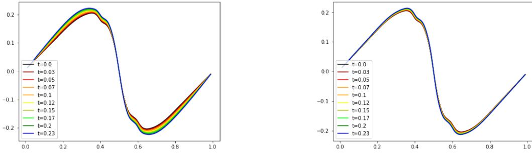
Figure 2.11: Numerical solution of piano string equation with  $V = \frac{1}{2}((1-g)u^2 + v^2) + (\frac{g}{2}(u^2v + \frac{1}{4}u^4))$ , where  $g = 0.783$ . Both pictures represent the piano string position in oscillation plane computed with reduce model and hyper-reduction built as in Figure 2.10. The parameter  $\alpha$  of the hyper-reduction is 0.00099 (left) and 0.00101 (right).
