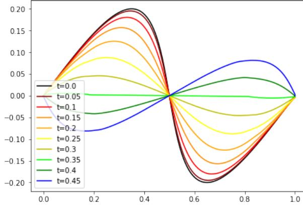
Figure 2.4: Numerical solution of piano string equation with  $V = \frac{1}{2}((1-g)u^2 + v^2)$ , where  $g = 0.537$  computed in high dimension with explicit Stormer-Verlet scheme, with  $n = 200$ ,  $dt = 0.0005$  and  $m = 500$ .
