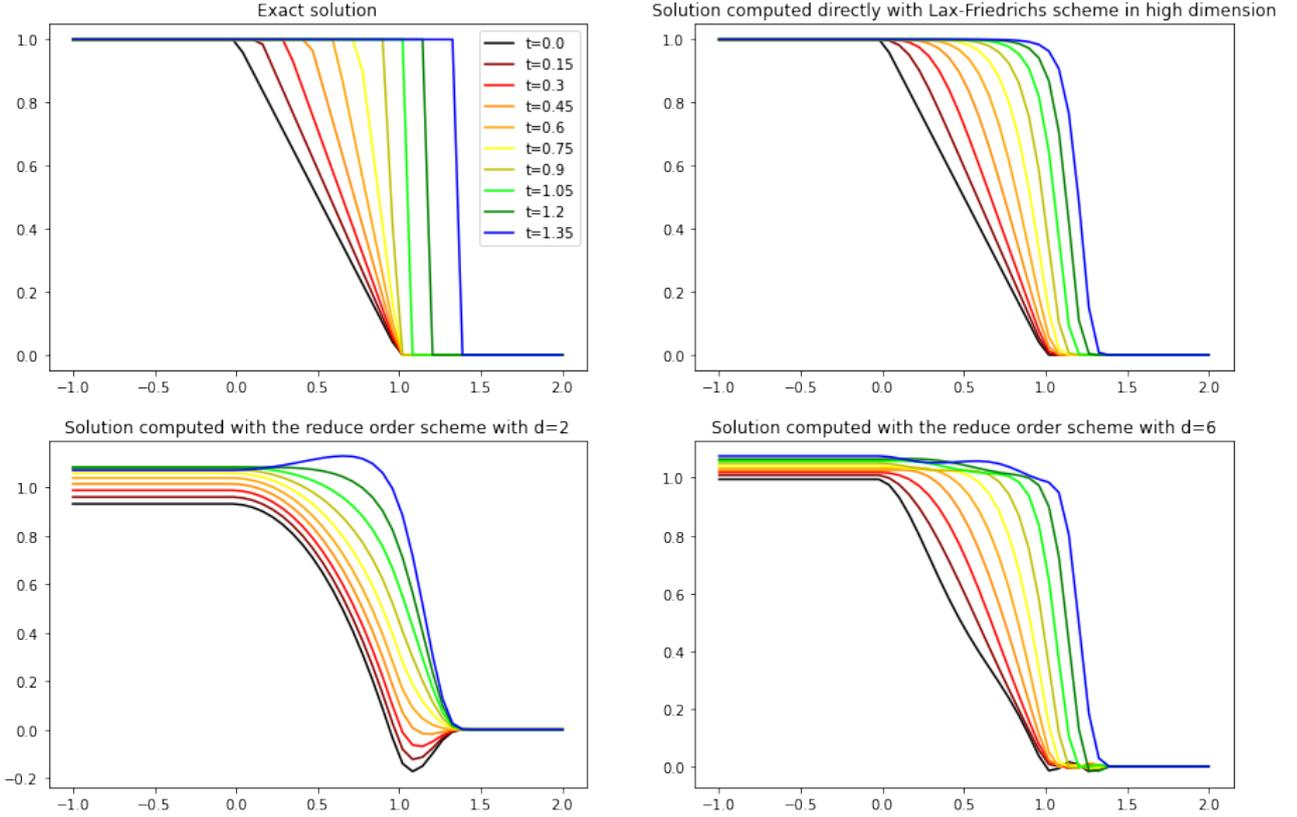
Figure 1.2: Numerical solution of Burgers' equation with  $\epsilon = 0$ . The solution obtained with the reduced order model with  $k = 2$  gives unaccurate results and with  $k = 6$ , it seems "noisy" for highest values of  $t$  next to singular points of the exact solution.
