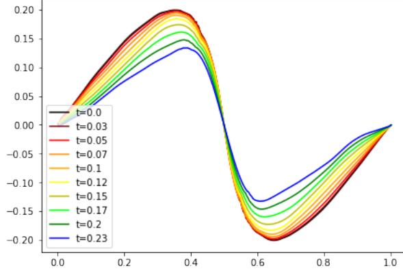
Figure 2.8: Numerical solution of piano string equation with  $V = \frac{1}{2}((1-g)u^2 + v^2) + (\frac{g}{2}(u^2v + \frac{1}{4}u^4))$ , where  $g = 0.8$  computed in high dimension with explicit Stormer-Verlet scheme, with  $n = 200$ ,  $dt = 0.0005$  and  $m = 500$ .
