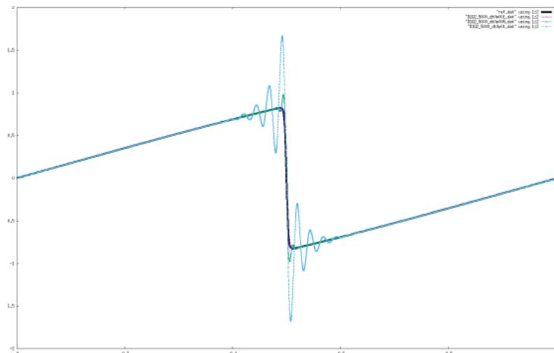
**Figure:** Comparison for different time step. Violet:  $\Delta t = 0.001$  (CFL 5-30), Green:  $\Delta t = 0.005$  (CFL 20-120), Blue  $\Delta t = 0.01$  (CFL 50-300), Black : reference
