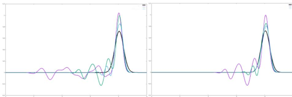
**Figure:** Left: comparison between different D1Q2 (violet  $M_a^0$ , green  $M_b^0$ , blue  $M_c^0$ , dark ref solution). Right: comparison between different D1Q3 (violet  $M_a^1$ , green  $M_b^1$ , blue  $M_c^1$ , dark ref solution)  $\Delta t = 0.2$ . (CFL  $\approx 200 - 500$ ).
