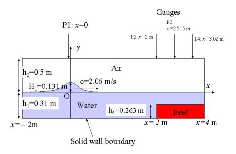
Figure 1. Boundary and initial conditions.
