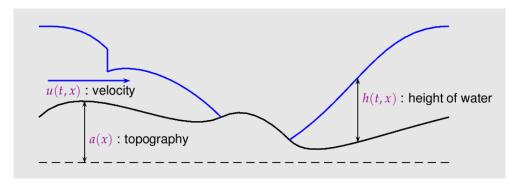
FIGURE 4. Description of the shallow-water model.
